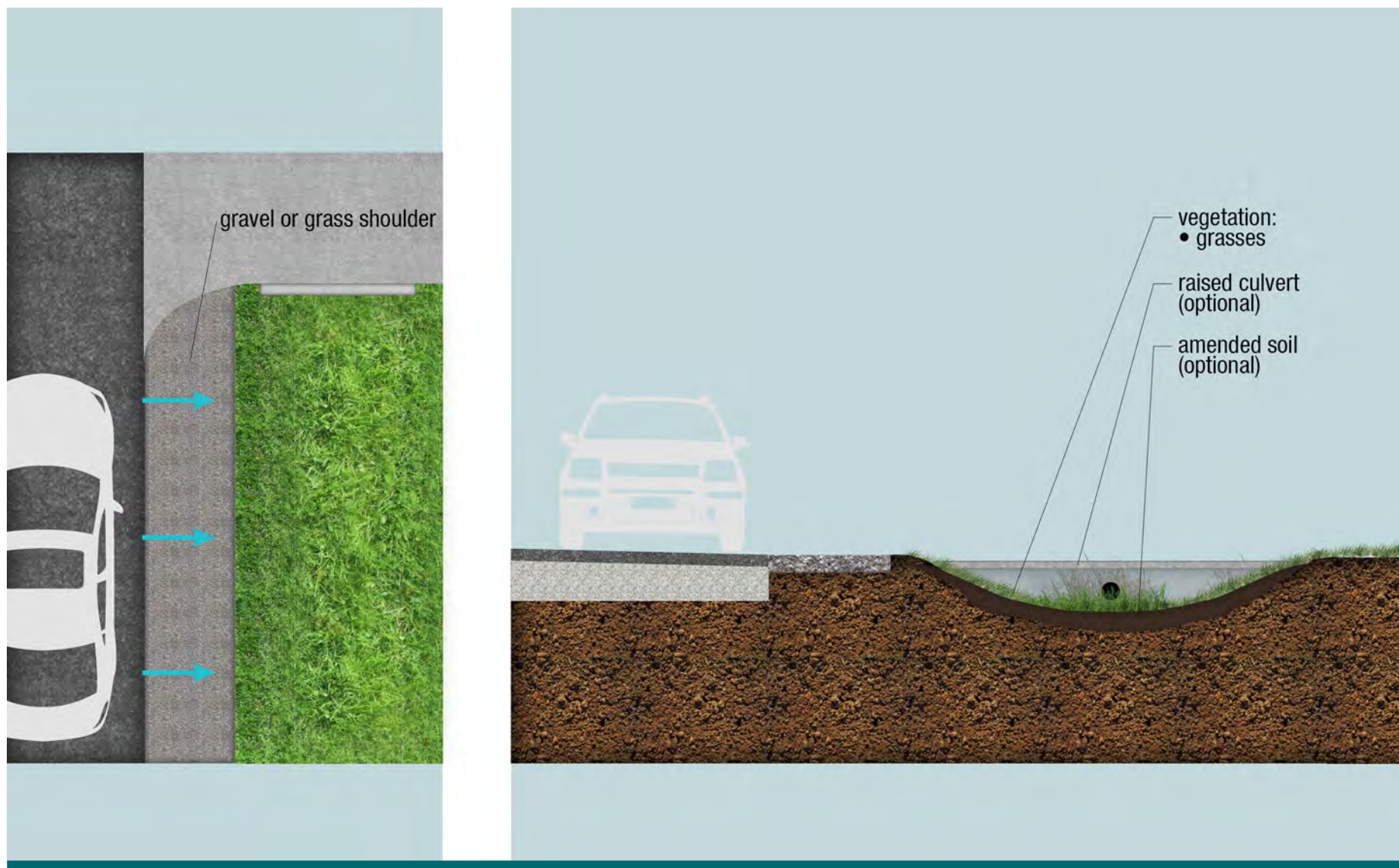
Figure 2.2.2: Enhanced grass swale plan view [left] and cross-section [right]
