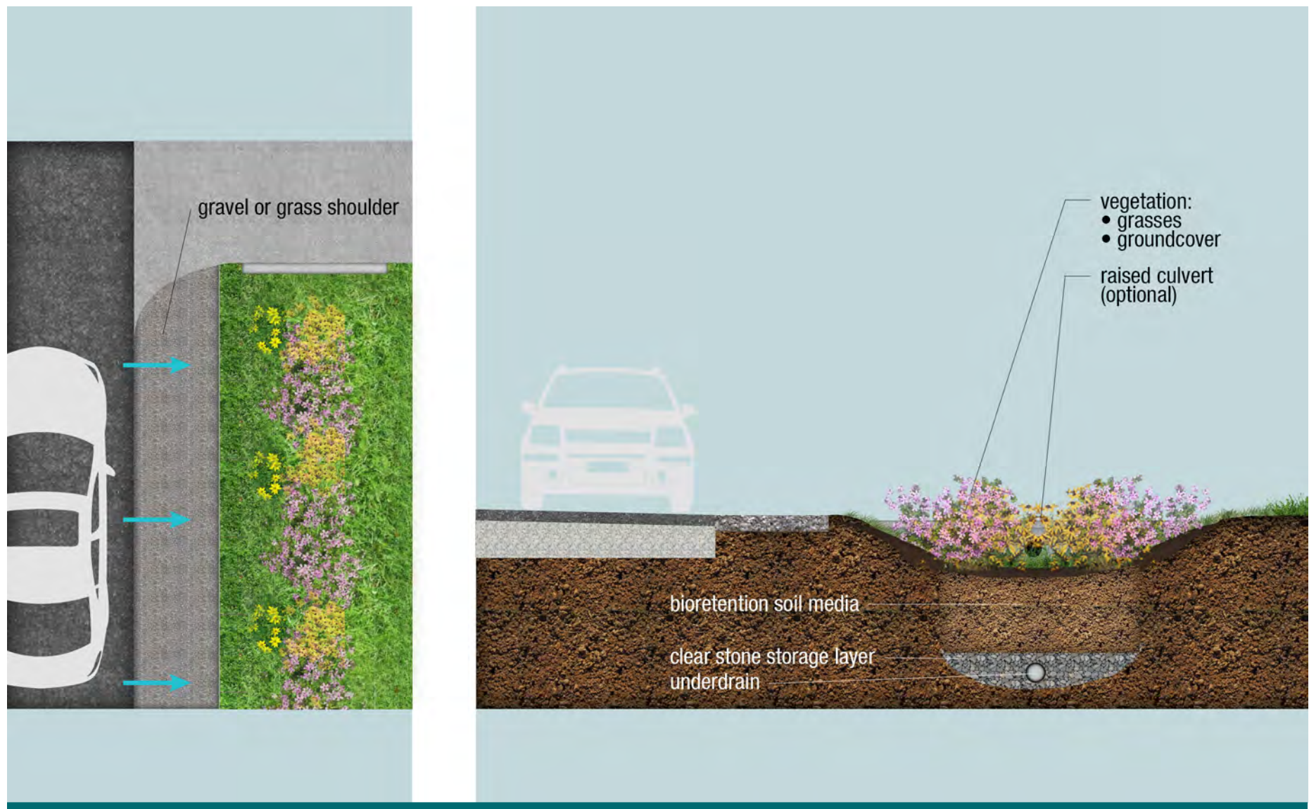
Figure 2.2.5: Bioswale plan view [left] and cross-section [right]
