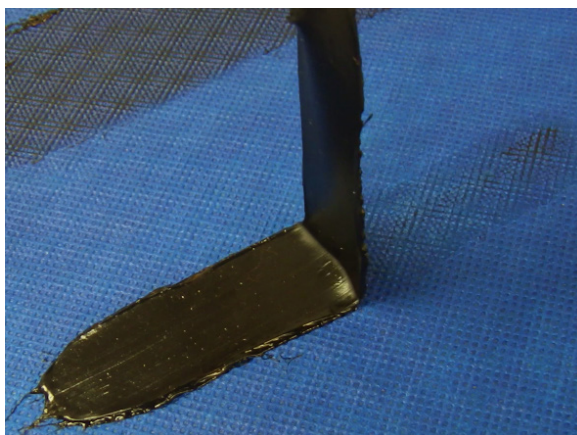
Sealant adhesion test showing adhesive failure from a synthetic vapour-permeable self-adhered membrane.
