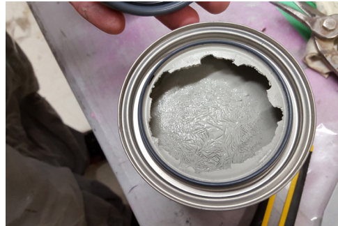
Liquid-applied membrane frozen due to extreme cold
